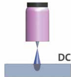
TIG DC half-wave: a high heat input into the workpiece is achieved.
